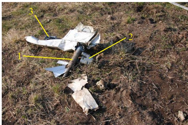
Fig. 11. Screw actuator for left wing flaps (1), electromagnetic brake ТЭМ-4 (2) and reducer (3). Photo taken by IAC (MAK) [8] Source: www.fakty-smolensk.gov.pl
