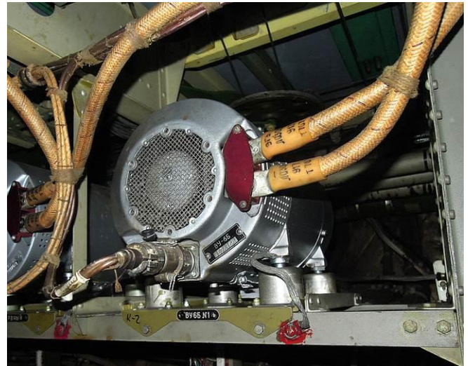
Fig. 5. Rectifier BY-6B 208 V 400 Hz/27 V DC on the Tu-154 aircraft. Source: http://commons.wikimedia.org/wiki/File:VU-6B-rectifying-device-on-Tu-154.jpg
