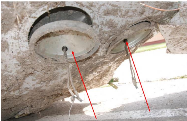
Fig. 17. Condition of landing/taxi lights PRF-4 mounted on the fuselage of the Tu-154M PLF101 after the crash. Photograph taken at the place of storage of the wreckage. Source: Annexure No 4 KBWL [6].
