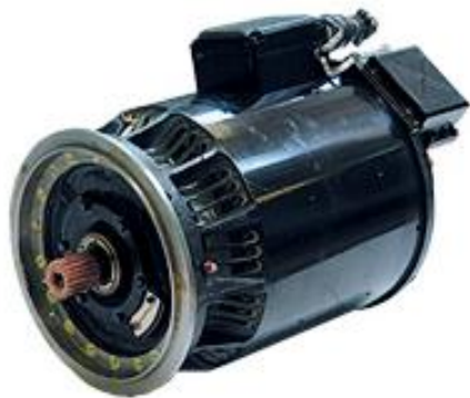
Fig. 3. Wound-field synchronous generator GT40PCh6.
