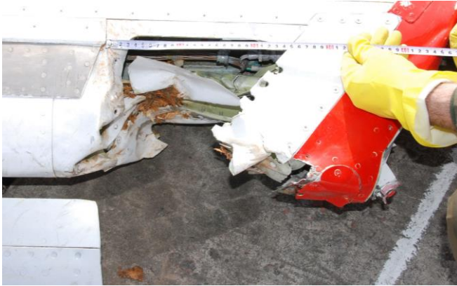
Fig. 20. A bundle of electric wires located before front spar of the detached portion of left wing. The front skin has been probably damaged when the severed part of wing hit the bushes at the crash site, while dropping. Note that slat covering the front skin has not been damaged Source: www.faktysmolensk.gov.pl [14 7].
