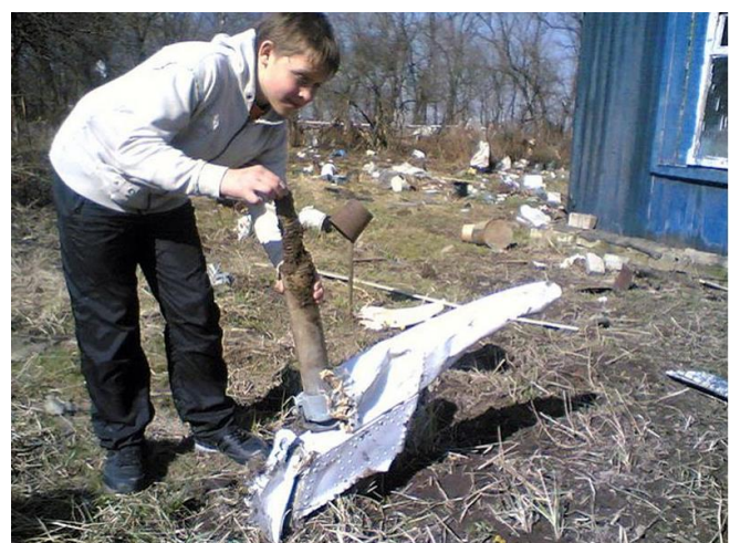
Fig. 10. Screw actuator of flaps found near N. Bodin's shed. Source: S. Amielin [10].
