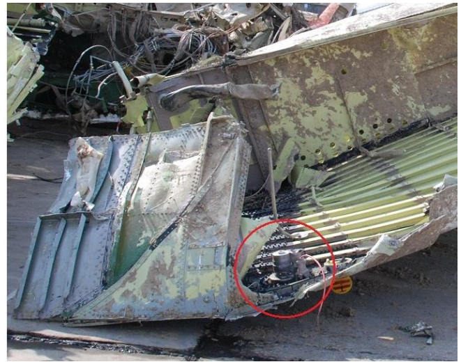
Fig. 18. Fuel booster pump ЭЦН-325 of the wing fuel tank in the left centerwing. Photograph taken at the place of storage of the wreckage. Source: www.fakty.molensk.gov.pl [7].
