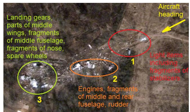
Fig. 1. The Tu-154M PLF 101 wreckage trail plot grouped by location of parts of the aircraft: (1) light items including fragments of stabilizers; (2) engines, fragments of middle and rear fuselage, rudder; (3) landing gears, parts of middle wings, fragments of middle fuselage, fragments of nose, spare wheels.
